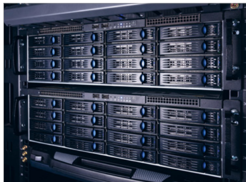
NAS (Network Attached Storage)
